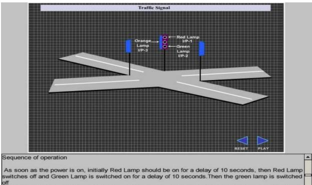
And Orange Lamp switches on for a delay of 2 seconds and then Red Lamp switches on and the cycle continues.
