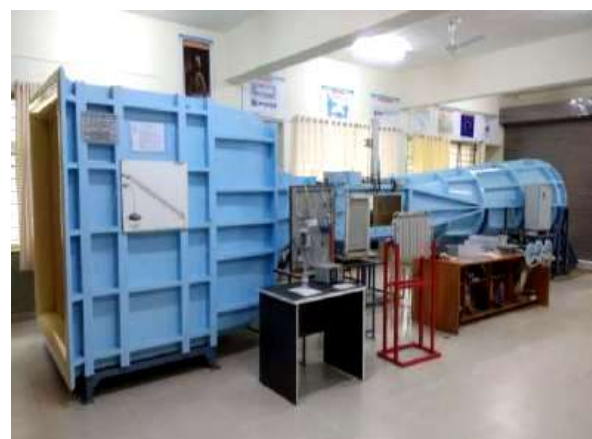
Figure 4. Photograph of the subsonic wind tunnel used in the present investigation.
