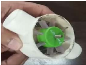
Fig.3: Turbine Enclosed in Casing
