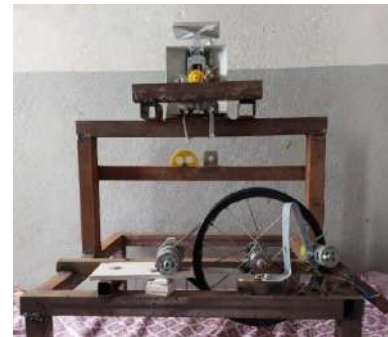
Fig. 8. Model of suspension and regenerative braking system
