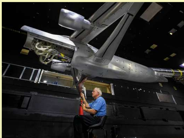
Instrumentation technician Michael Hodgins performs installation measures on the trans-sonic truss-braced wing model at Langley Research Center's 14x22 subsonic wind tunnel.
